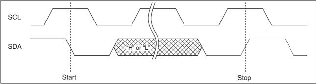
Note : At the write operation, the FRAM device does not need the programming wait time (twc) after issuing the Stop Condition.
