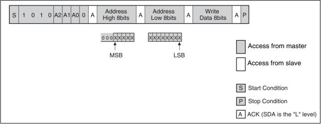
Note : In the MB85RC64TA, input "000" as the upper 3 bits of the MSB.
